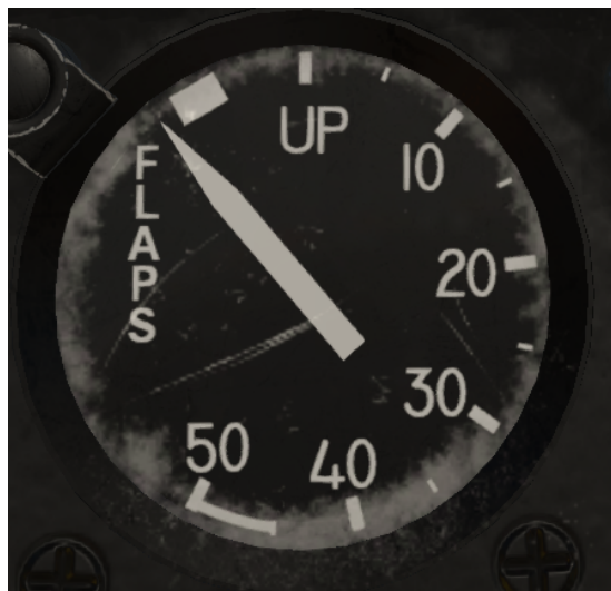
Figure 23: Flaps indicator represented with no power supplied
