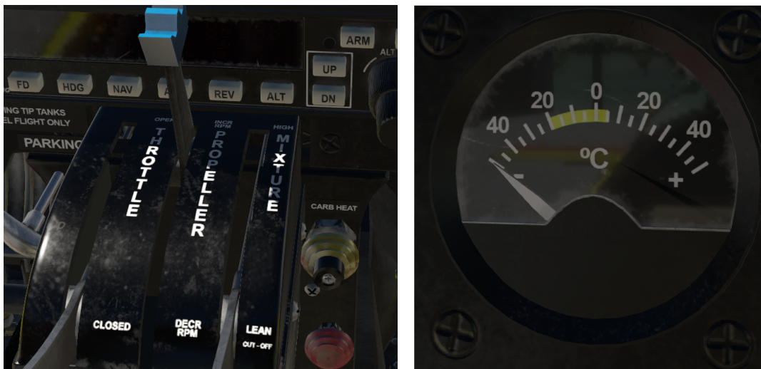
Figure 15: Left: the carburetor heat knob is labelled CARB HEAT. Right: carburetor temp gauge
