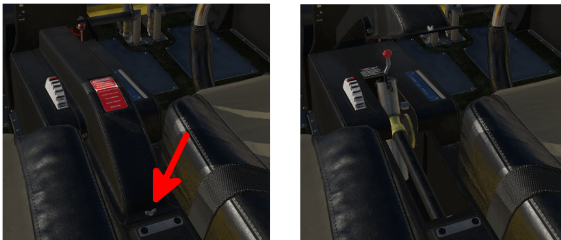
Figure 22: Click in the position indicated by the arrow pointer to remove the handle cover
